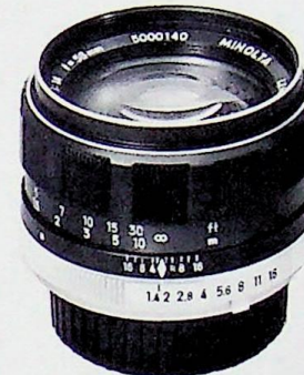
58mm MC Rokkor: F1.4 Lens elements: 6 elements in 5 groups Angle of view: 41° Focus: to 2 feet / 0.6 meters Filter screw diameter: 55mm Diaphragm: Auto pre-set F1.4—F16
