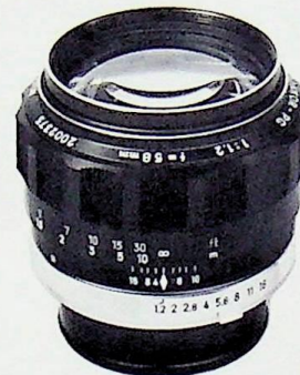
58mm MC Rokkor: F1.2 Lens elements: 7 elements in 5 groups Angle of view: 41° Focus: to 2 feet / 0.6 meters Filter screw diameter: 55mm Diaphragm: Auto pre-set F1.2—F16
